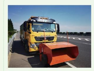
Quick Pickup and Collection Device for Highway Litter
