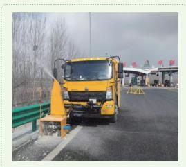
Operation of High-Speed Snow Removal Equipment for Highway Shoulders
